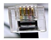
Picture 1: RJ11 connector (four lines inside)
