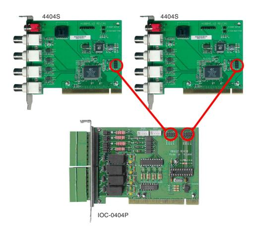
2. IOC-0404P to 4404Q: Take note that the red line of the cable should connect to Pin2 on the IOC-0404P card and to the "G" pin on the 4404Q card.
