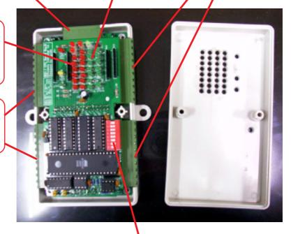
RS232/RS485 Communication Port, and Communication IP (DIP Switch)
