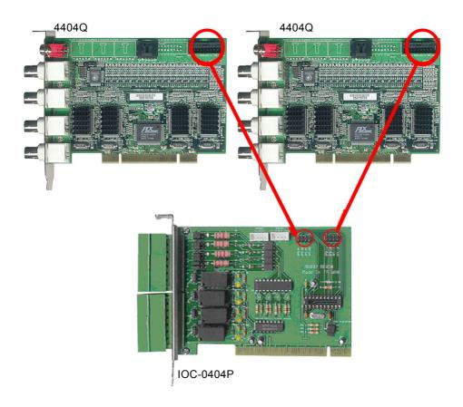
3. IOC-0404P to 4408QB: Take note that the red line of the cable should connect to Pin2 of the IOC-0404P card and to the "G" pin on the 4408QB card.
