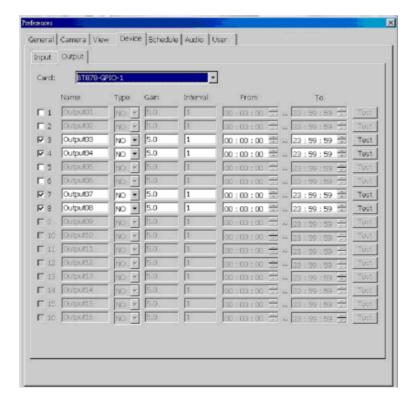
**Note:** If IO-0404P connects to two capture cards, the number of output pins are 8. They are output 3, 4, 7, 8, 11, 12, 15 and 16.
