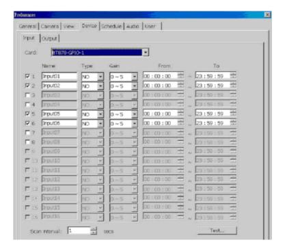
Note: If IO-0404P connects to two capture cards, the number of input pins are 8. They are input 1, 2, 5, 6, 9, 10, 13 and 14.
