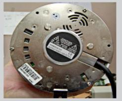
Picture 2: Jumpers at the bottom side of PZT camera base
